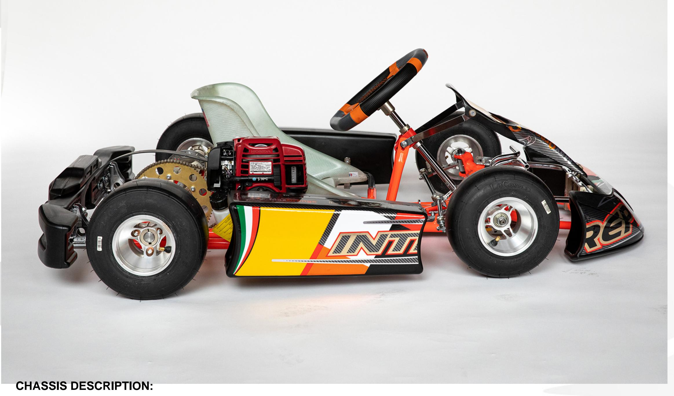
Chassis made to suit children from 5 to 7 years old. Suitable for all types of stature thanks to special technological and innovative mechanisms that allow changing the position of both the seat and the pedals.
